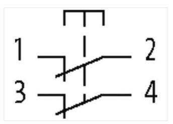
Male PIN 1: N/C1 PIN 2: N/C1 PIN 3: N/C 2 PIN 4: N/C 2
